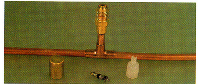
Figure 45-124 Full-size gage connections must be installed to remove moisture. Photo by Bill Johnson
