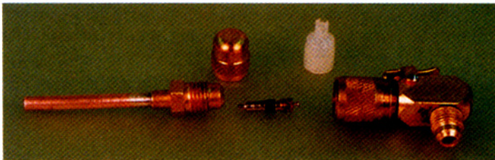
Figure 45-84 Remove the Schrader valve depressors from gage lines and use the special fitting on the right to depress the valve cores. Photo by Bill Johnson
