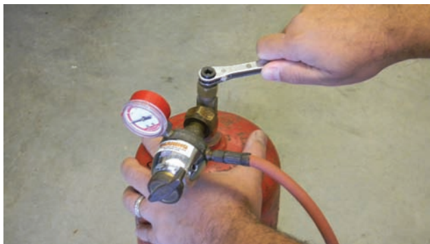
Figure 7.28 The proper procedures for setting up, lighting, and using an air-acetylene torch.
