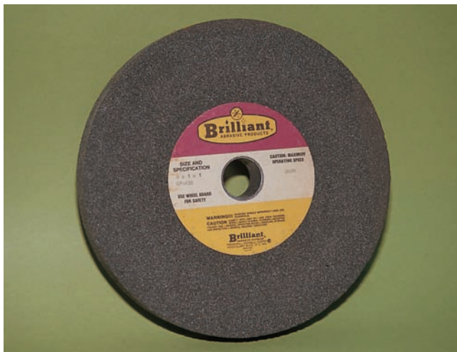
Figure 4.32 When installing a grinding stone, ensure that it is compatible with the grinder.
