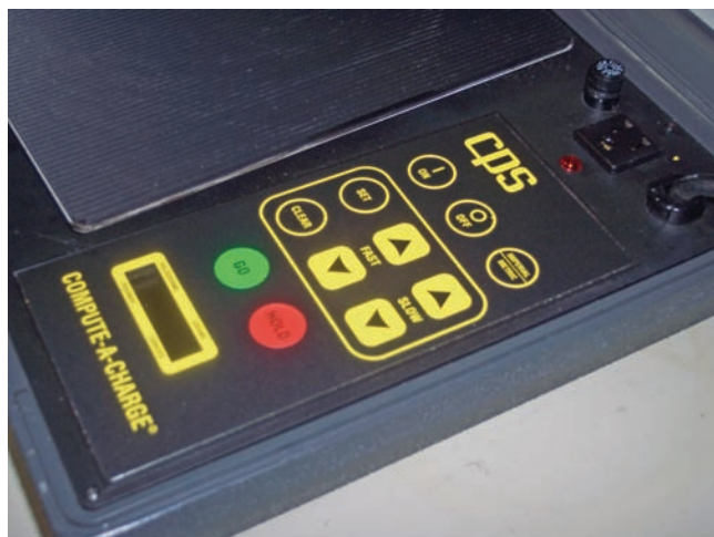
Figure 10.13 Automatic charging scales can be programmed to charge a precise quantity of refrigerant into the system. Photo by Eugene Silberstein
