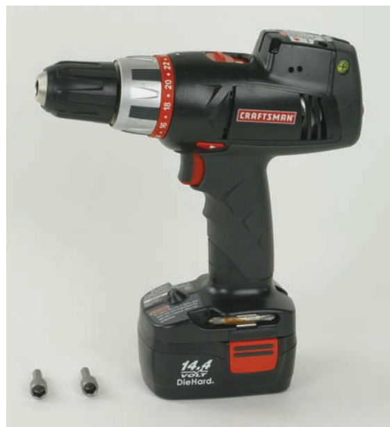
Figure 36.34 A portable electric drill and screw holders.
