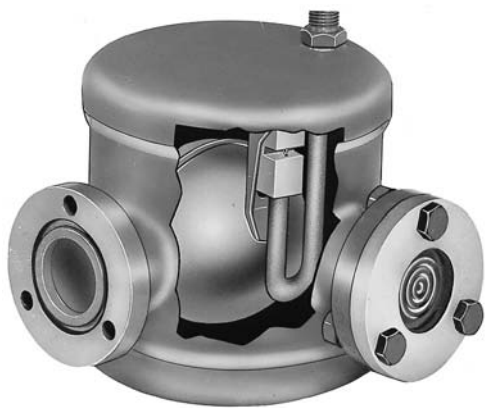
Figure 26.19 A compressor float-operated oil-level regulator. Courtesy AC & R Components, Inc.
