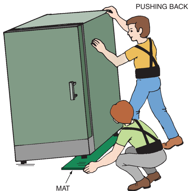
Figure 45.123 Enough room is available to tilt the box and place a mat under the feet.
