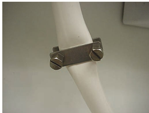
Figure 27.23 A restrictor in the water line from the water pump allows for varying the water flow rate. Courtesy Ferris State University. Photo by John Tomczyk
