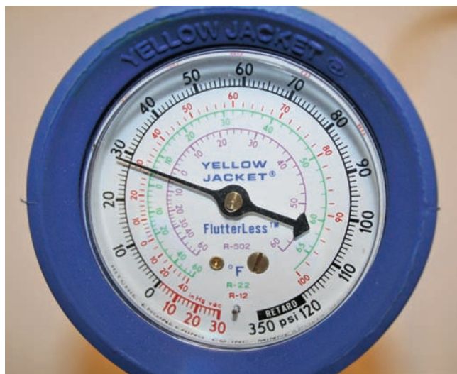
Figure 21.6 Many pressure gauges have temperature/pressure relationships printed on the gauge.
