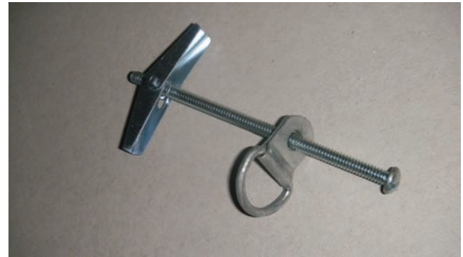
Figure 6.19 Make certain that the item being secured is placed on the bolt before the toggle is screwed onto the bolt. Photo by Eugene Silberstein
