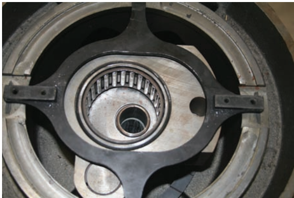
Figure 23.50 A scroll compressor's drive train showing center bearing and motor shaft offset. Courtesy Ferris State University. Photo by John Tomczyk
