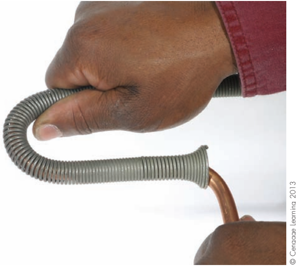
Figure 7.14 Tube bending springs are used to help prevent kinking the tubing while bending. Be sure to use the proper size.
