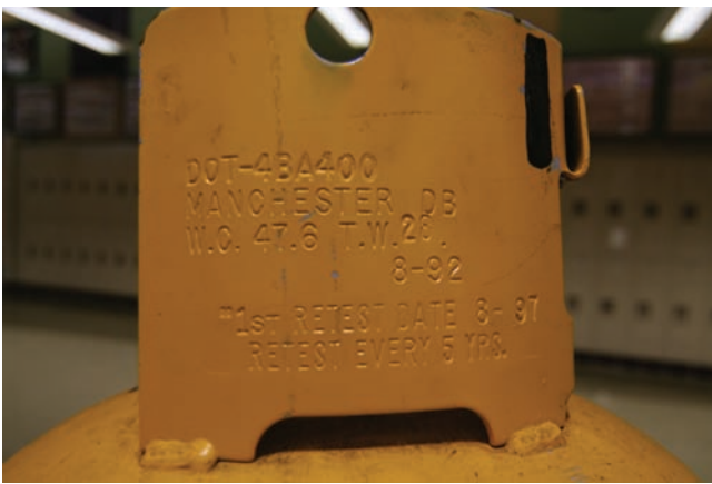
Figure 9.34 Refrigerant recovery tank specifications stamped on the protective head of the tank, showing tare weight and water capacity. Courtesy Ferris State University. Photo by John Tomczyk
