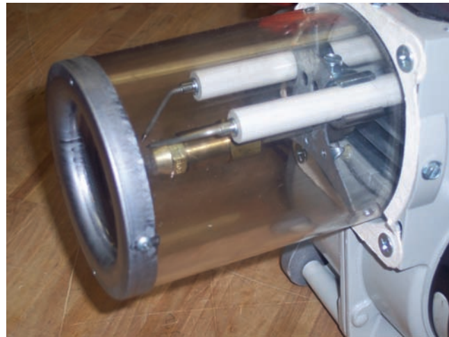
Figure 32.57 Hollow air tube showing placement of the nozzle and electrodes in the tube. The hollow tube is for illustrative purposes only. Courtesy Oilheat Associates, Inc. Photo by John Levey
