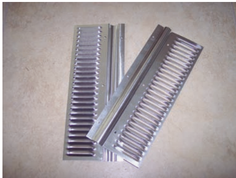
Figure 33.101 Aluminum "fins" used to increase the heat transfer surface of the PEX tubing in a dry, concrete-free radiant application.
