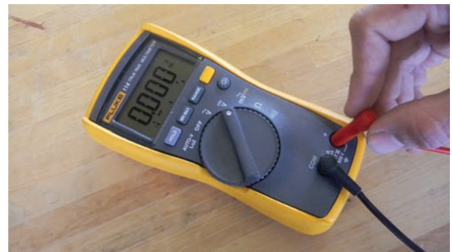
Figure 12.44 Plugging the test leads into the VOM. Photo by Eugene Silberstein
