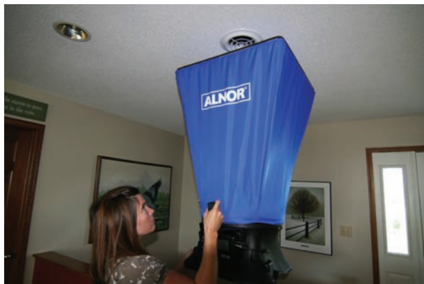
Figure 39.68 A residential energy auditor using a flow hood to measure the airflow (cfm) out of a ceiling diffuser in a residence.
