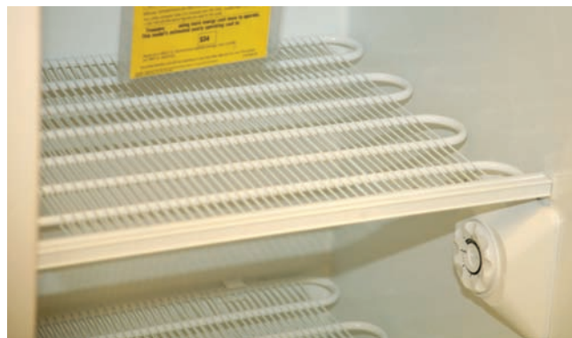
Figure 45.49 Shelf-type evaporators are normally steel tubing with wire to add support. Photo by Bill Johnson
