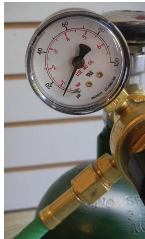
Figure 7.37 This oxygen regulator gauge indicates 10 psig.
