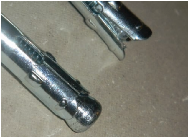
Figure 6.16 Image showing the anchor shield before and after expansion. Photo by Eugene Silberstein
