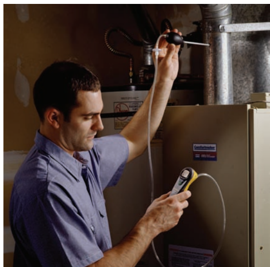
Figure 39.52 A technician testing the ppm carbon monoxide (CO) in a furnace's flue gases. Courtesy Fluke Corporation
