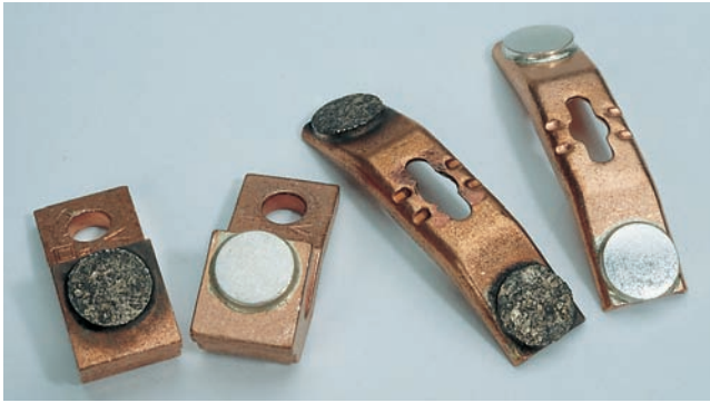
Figure 47.80 New and old sets of contacts. The old ones are pitted from many motor starts. Courtesy Square D Company
