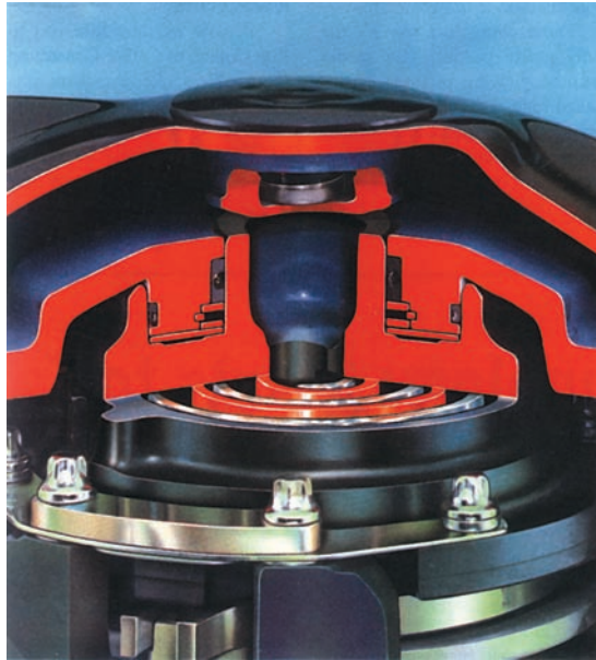
Figure 23.49 Two spiral-shaped scrolls fitting inside one another. Courtesy Emerson Climate Technologies
