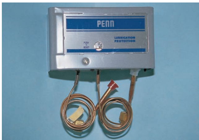
Figure 25.30(A) Oil safety controls have a bellows on each side. They are opposed in their forces and measure the net oil pressure: the difference in the suction pressure (oil pump inlet) and the oil pump outlet pressure. This control has a 90-sec time delay to allow the compressor to get up to speed and establish oil pressure before it shuts down.
