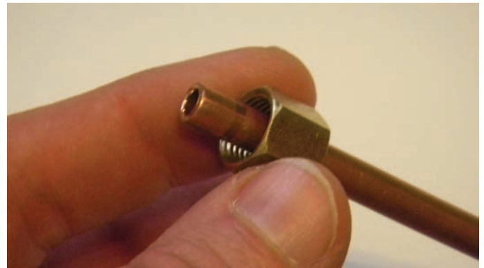
Figure 7.57 Placing the compression nut on the tubing.
