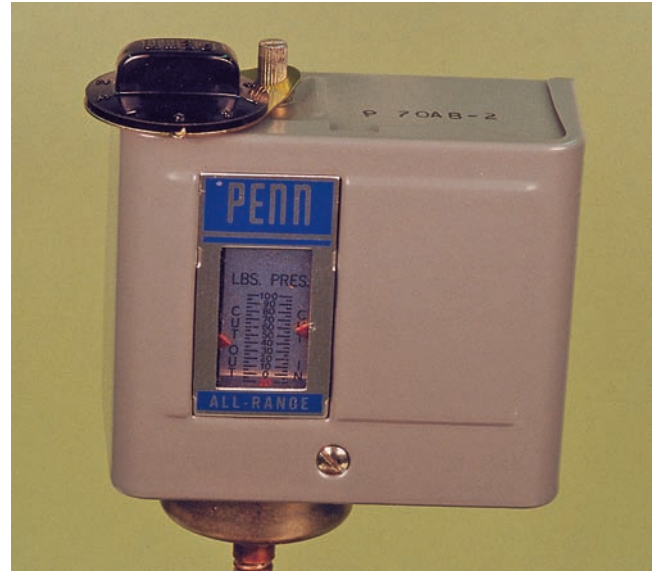
Figure 25.23 The low-pressure control. The control contacts close on a rise in pressure and open on a fall in pressure. If the low-side pressure goes below the control's set point, the control will open its contacts to the compressor's control circuit. Photo by Bill Johnson
