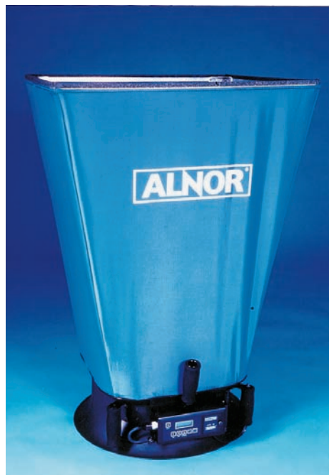
Figure 37.87 This hood fits directly over ceiling registers up to about 2 ft × 2 ft. The hood forces the air from the register through the meter and displays the airflow in cfm. Courtesy Alnor Instrument Company
