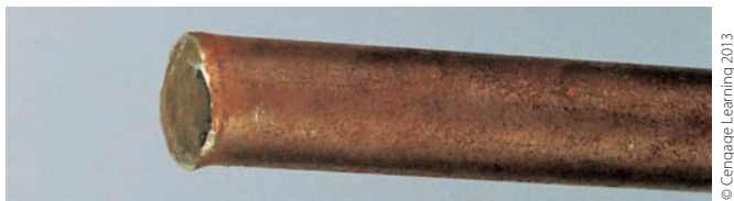
Figure 20.5 A motor shaft damaged from trying to drive it through the pulley. Photo by Bill Johnson
