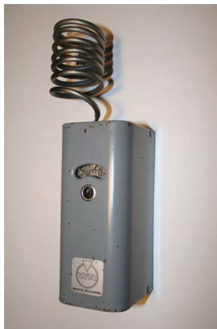
Figure 14.14 The line-voltage thermostat used to stop and start a compressor that draws up to 20 A full-load current and has an inrush current of up to 80 A. Courtesy Ferris State University. Photo by John Tomczyk
