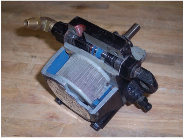
Figure 32.44 Cutaway view of an oil pump showing the screen. Courtesy Oilheat Associates, Inc. Photo by John Levey
