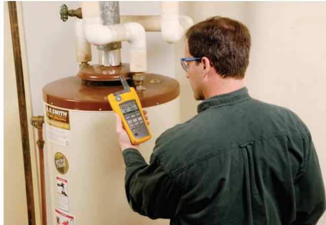
Figure 5.75 A technician checking a water heater for carbon monoxide spillage with a digital multi-parameter air testing instrument. Courtesy of Fluke Corporation
