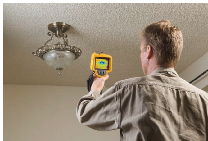
Figure 39.15(A) An auditor aiming a thermal imaging camera at a light fixture. Courtesy Fluke Corporation
