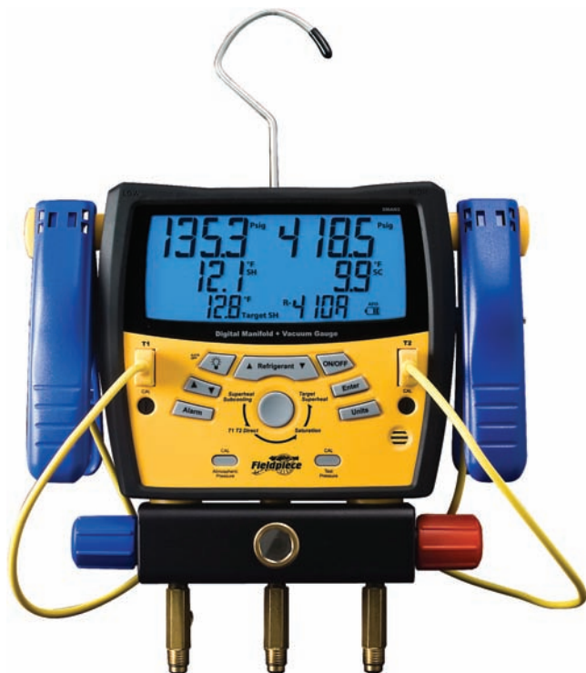
Figure 41.1(B) A modern digital gauge manifold set with temperature measuring probes for measuring superheat and subcooling. This gauge set also has pressure/temperature relationships of different refrigerants resident in its memory. Courtesy Fieldpiece Corporation
