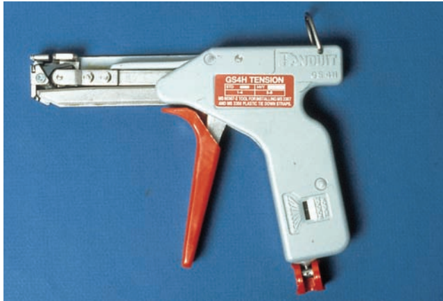
Figure 5.48 A tool used to install nylon strap clamps around a flexible duct. Photo by Bill Johnson
