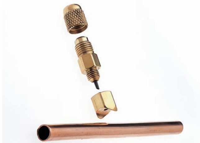
Figure 25.59 This valve can be soldered on a vapor line while the system has pressure in it. Low-temperature solder is used. It cannot be soldered to a line with liquid in it because the liquid will not allow the line to get hot enough. Courtesy J/B Industries
