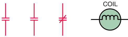
Figure 19.5 A relay with two sets of contacts that close and one set of contacts that opens when the coil is energized. It has two normally open (NO) sets and one normally closed (NC) set. © Cengage Learning 2013
