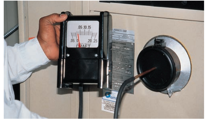
Figure 32.98 Checking overfire draft. Photo by Bill Johnson
