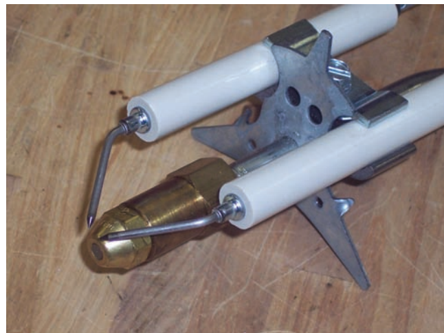
Figure 32.58 Electrode location with respect to the nozzle. Courtesy Oilheat Associates, Inc. Photo by John Levey
