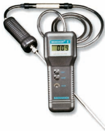
Figure 34.5 A testing device that will measure ppm of carbon monoxide. Courtesy Bacharach, Inc., Bacharach Institute of Technical Training
