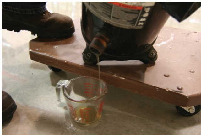
Figure 8.61 (A) Soot and sludge move into the condenser when a motor burn occurs while the compressor is running. (B) Oil being drained from a fully hermetic compressor which has had a motor burn. (C) An acid test kit used for checking the acidity of compressor oil after a suspected motor burn. (D) A combination sight glass and moisture indicator for installation in the liquid line after the filter drier.
