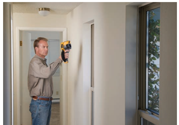
Figure 39.11(C) An energy auditor taking a thermal image on the interior of a window and the surrounding window framing. Courtesy Fluke Corporation
