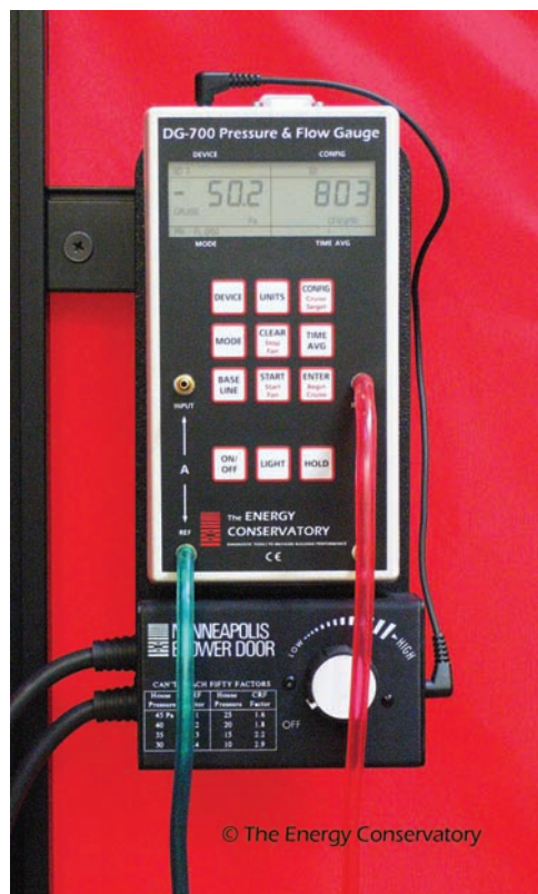
Figure 39.8 Blower door instrumentation, which includes digital gauges like manometers and anemometers that measure the flow of air through the blower door's fan at a set pressure differential between the inside and outside of the house. Courtesy The Energy Conservatory
