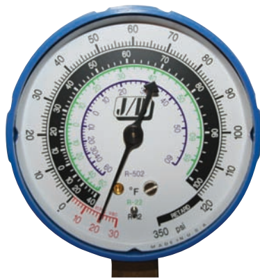
Figure 8.38 Manifold gauge reading 20 in. Hg vacuum. Courtesy Ferris State University. Photo by John Tomczyk
