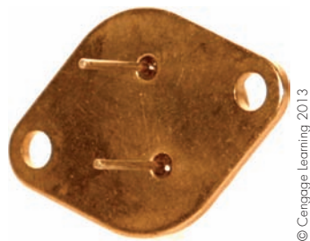
Figure 17.48 This power transistor is basically an electronic switch that does not arc when it changes position and has the ability to turn on and off very quickly.
