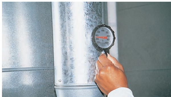
Figure 32.102 Making a stack gas temperature test. Photo by Bill Johnson
