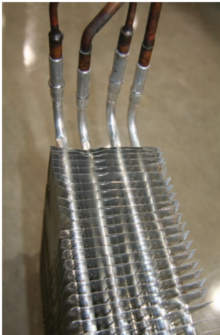
Figure 21.16 (A) A multicircuit evaporator fed with a distributor to reduce pressure drop. (B) and (C) A two-pass, multicircuit, finned-tube evaporator. There are actually two evaporators in parallel to reduce pressure drop. (A) Courtesy Sporlan Valve Company. (B) and (C) Courtesy Ferris State University. Photos by John Tomczyk
