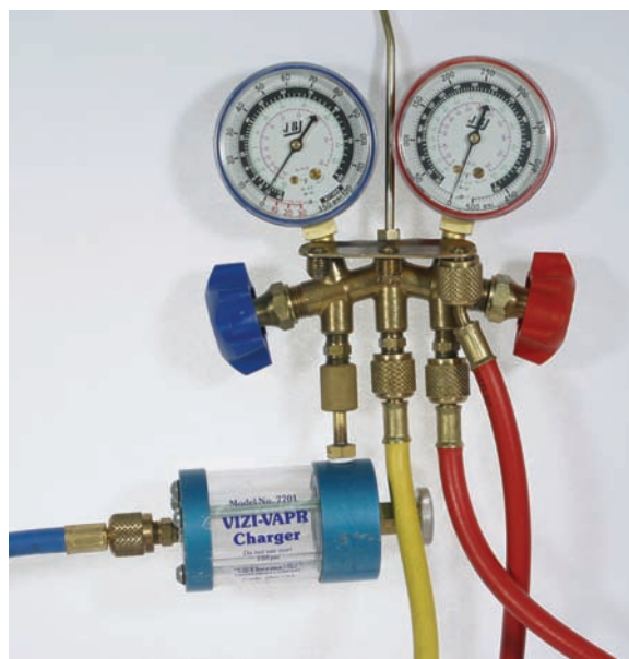
Figure 10.10 A charging device in the gauge line between the liquid refrigerant in the cylinder and the suction line of the system.
