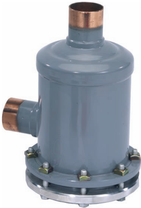
Figure 25.42(C) This suction filter has a removable core. Its casing or shell is left in the system and only the core is replaced, once the system is pumped down, by removing the bolts and end cap. Filters can be filters only or a combination of a filter and a drier, depending on the makeup of the core. Courtesy Sporlan Division, Parker Hannifin Corporation
