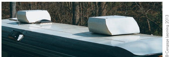
Figure 46.6 A roof-mount unit for recreational vehicles. Sometimes these are used in small stand-alone buildings. Photo by Bill Johnson
