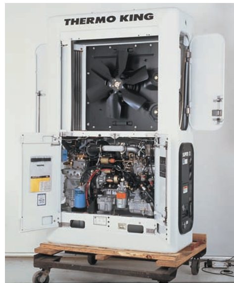
Figure 28.13 Access for service to a nose-mount unit. Courtesy Thermo King Corp.
