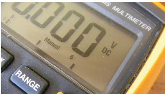
Figure 12.42 6 VDC range on the VOM. Photo by Eugene Silberstein
