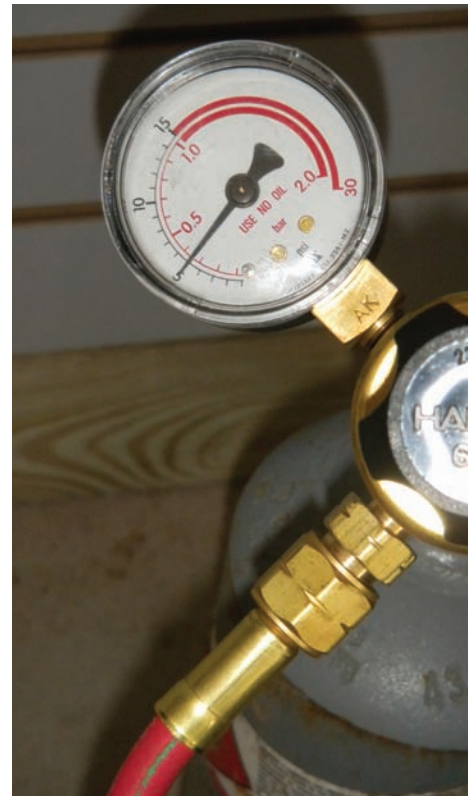
Figure 7.36 The acetylene regulator gauge indicates 5 psig.
