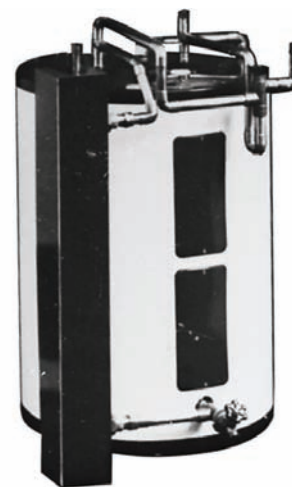
Figure 22.51 A heat exchanger to capture the heat from the highly superheated discharge line and use it to heat domestic water. This line can easily be 210°F and can furnish 140°F water in a supply limited by the size of the refrigeration system. The larger the system, the more heat is available. Courtesy Noranda Metal Industries, Inc.
