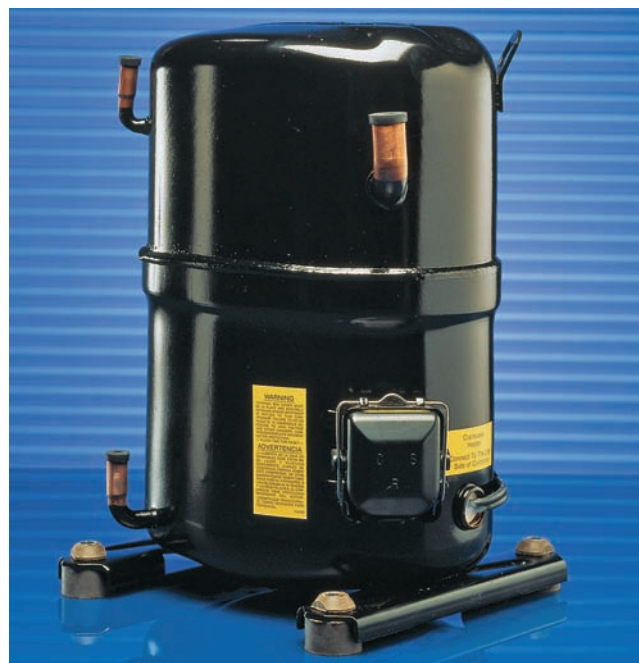
Figure 23.11 The welded hermetic compressor is typical of smaller compressors, from fractional horsepower to about 50 hp. In most welded hermetic compressors, the suction line is usually piped directly into the shell and is open to the crankcase. The discharge line is normally piped from the compressor inside the shell to the outside of the shell. The compressor shell is typically thought of as a low-side component. Courtesy Bristol Compressors, Inc.
