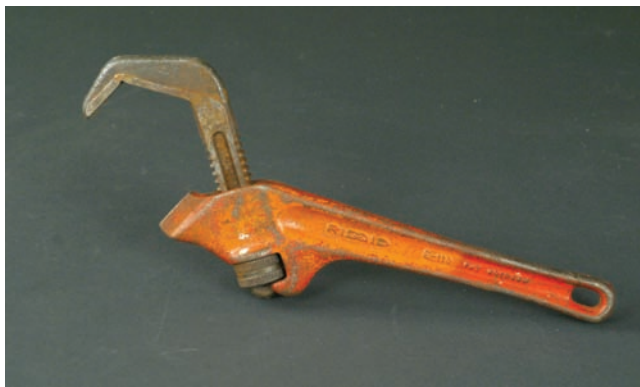
Figure 49.14 This wrench can be used to remove valve stem caps. Photo by Bill Johnson
