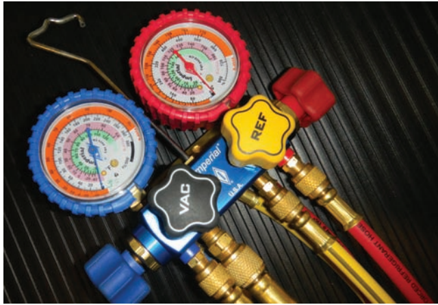
Figure 1.2 Pressure gauge used to measure the system operating pressures in air-conditioning and refrigeration equipment. Photo by Eugene Silberstein
