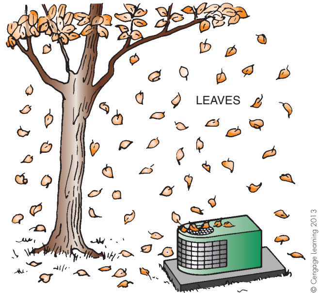
Figure 36.31 In units that discharge air from the top, the fan is usually on the top.
