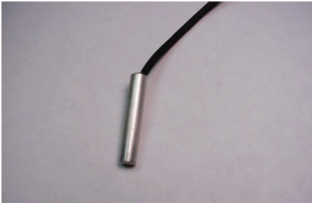
Figure 24.37 A thermistor used as a temperature sensor for the controller input. Courtesy Ferris State University. Photo by John Tomczyk.
