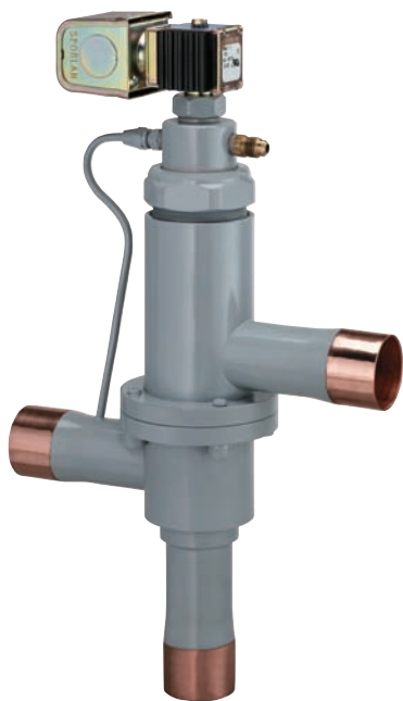
Figure 26.6 This three-way heat reclaim valve is pilot operated and solenoid activated. Courtesy Sporlan Division, Parker Hannifin Corporation
