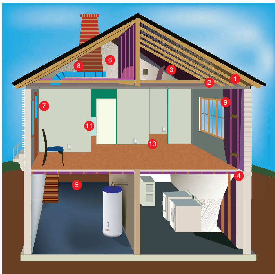
Figure 39.9 Air leakages into a residential structure using a blower door test. Courtesy The Energy Conservatory
