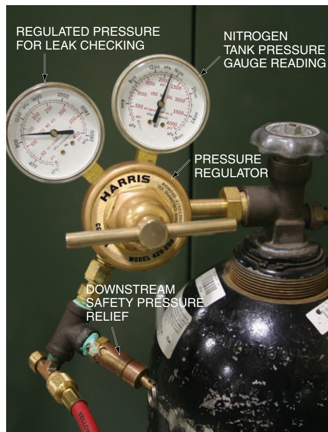
Figure 4.9 A nitrogen tank with pressure regulator and safety downstream pressure relief valve.
