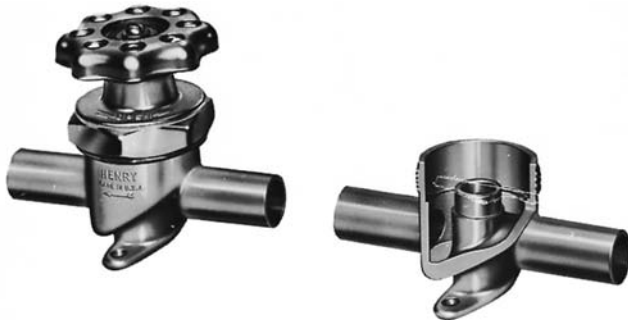
Figure 25.54 The diaphragm hand valve used when servicing a system. This valve is either open or closed, unlike the suction and discharge valves with a gauge port. The valve has some resistance to fluid flow, called pressure drop. It can be used anywhere a valve is needed. The larger sizes of this valve are soldered into the line. Care should be taken that the valve is not overheated when being soldered.
