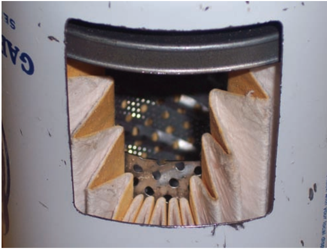
Figure 32.20 Cutaway view of an oil filter. Courtesy Oilheat Associates, Inc. Photo by John Levey
