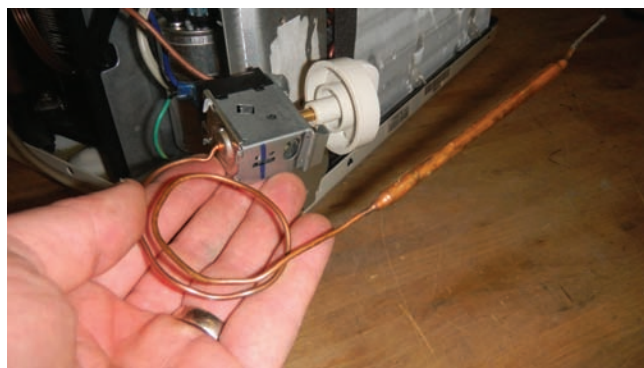
Figure 14.13 The window air conditioner has a line-voltage thermostat that starts and stops the compressor. On some models with energy-saving modes, the thermostat cycles both the compressor and the fan motor. Photo by Eugene Silberstein
