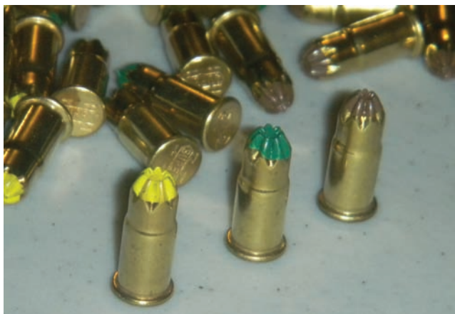
Figure 6.37 Color-coded powder loads. Photo by Eugene Silberstein
