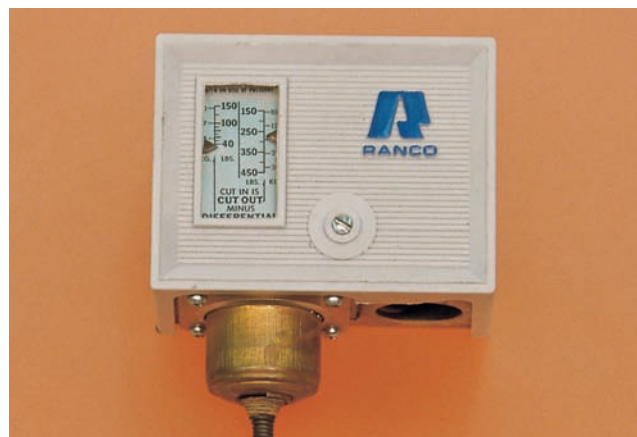
Figure 22.37 A condenser fan-cycling device. This control performs the same action (make on a rise in pressure) as the low-pressure control except that it operates at a much higher range. Photo by Bill Johnson
