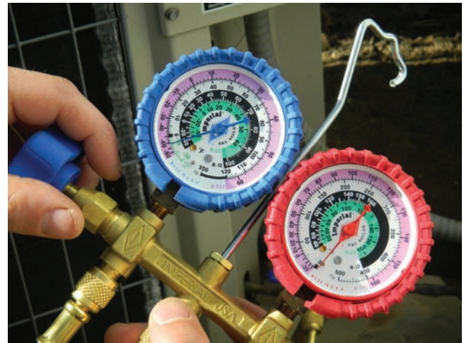
Figure 1.24 The gauge on the left, called a compound gauge , reads pressures above and below atmospheric pressure. The gauge on the right, called the high-pressure (high-side) gauge , will read up to 500 psi.
