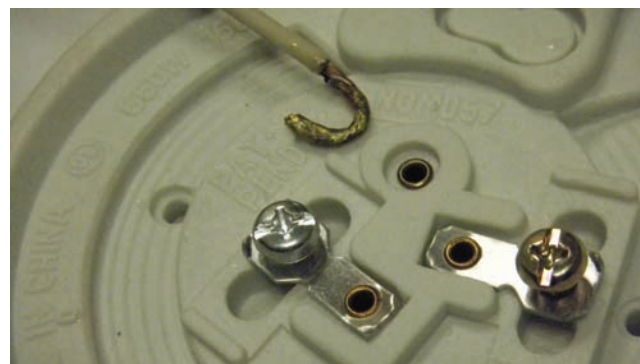
Figure 6.49 The tinned wire being secured under a screw terminal. Photo by Eugene Silberstein
