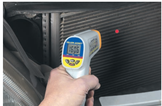
Figure 5.36 (A) Digital thermometer, (B) infrared thermometer, (C) infrared thermometer measuring a coil temperature.
