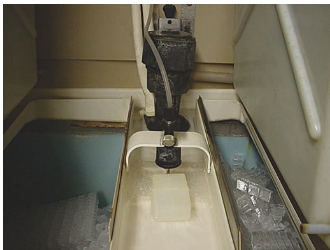
Figure 27.28 A water reservoir, float mechanism, incoming water line, and water pump. Courtesy Ferris State University. Photo by John Tomczyk
