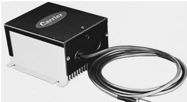
Figure 25.16(A) A control used to vary the fan speed on a special motor based on condenser temperature. Courtesy Carrier Corporation
