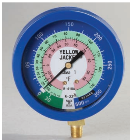
Figure 41.2(C) A gauge designed to handle the higher pressures of R-410A. Courtesy Ritchie Engineering Company, Inc.
