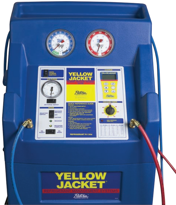
Figure 9.18 A modern refrigerant recycling and recovery machine showing sophisticated control panel.
