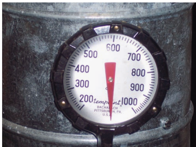
Figure 11.2 The thermometer is included in the flue-gas analysis kit. Note the high temperature range of the thermometer.
