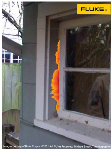
Figure 39.27 A thermal imaging camera showing warm air exfiltrating around the side of a window. Courtesy Fluke Corporation
