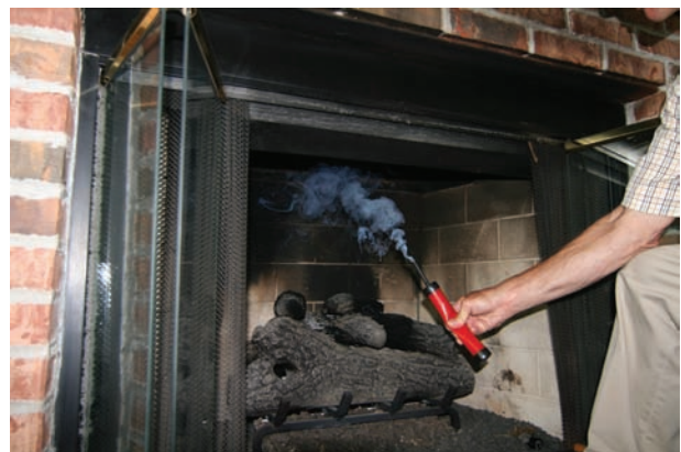
Figure 39.55(C) A technician checking for backdrafting in a residential fireplace using a chemical smoke generator.
