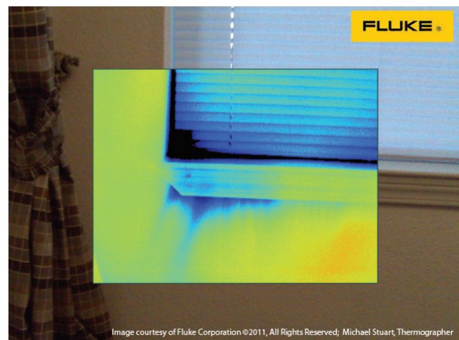
Figure 39.19 A thermal imaging camera showing cold air infiltration around a window. Courtesy Fluke Corporation
