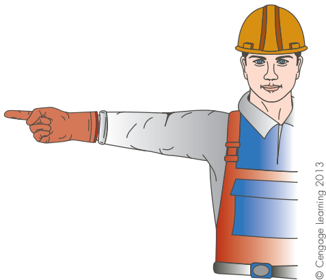
Figure 50.23 By an extended arm and a pointed finger, the crane operator knows which way to rotate the boom.
