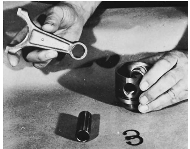
Figure 23.25 The end of the rod that fits into the piston. The wrist pin holds the rod to the piston while allowing the pivot action that takes place at the top of the stroke. The wrist pin is held secure in the piston with snaprings. Courtesy Trane Company 2000
