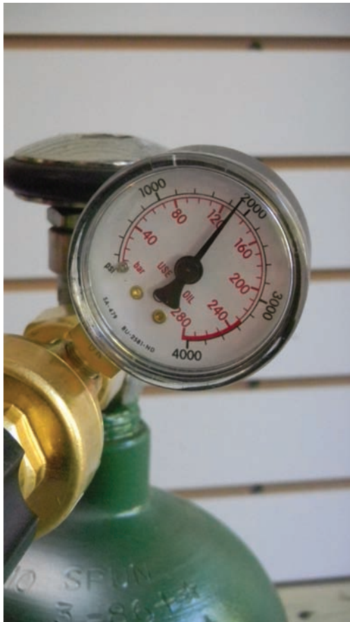
Figure 7.35 Pressure registers on the oxygen cylinder gauge.
