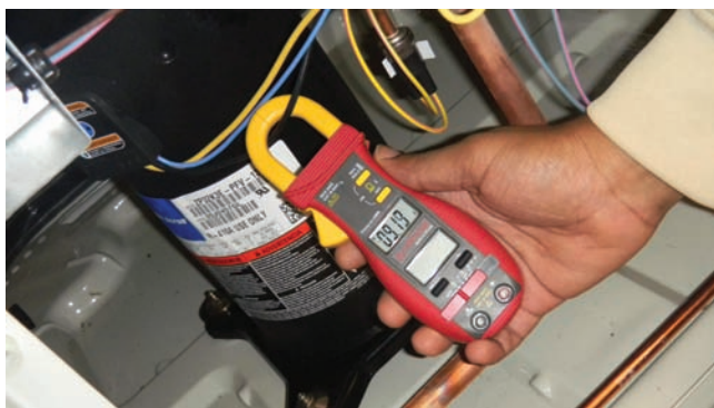
Figure 12.46 Measuring amperage by clamping the jaws of the meter around the conductor. Photo by Eugene Silberstein
