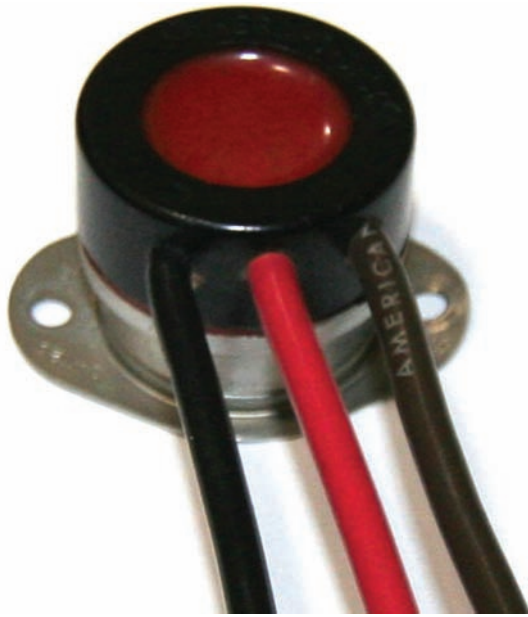
Figure 25.37 A sensor used with the timer in Figure 25.36 . The sensor has three wires and is a single-pole–double-throw device. It has a hot contact (made from the common to the terminal that is energized on a rise in temperature) and a cold contact (made from the common to the terminal that is energized when the coil is cold). This control is in either the hot or the cold mode. It is often referred to as a defrost termination and fan delay (DTFD) switch. Courtesy Ferris State University. Photo by John Tomczyk
