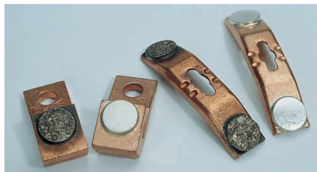
Figure 19.15 Clean contacts contrasted with a set of dirty, pitted contacts. Courtesy Square D Company
