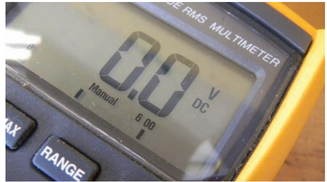
Figure 12.43 600 VDC range on the VOM. Photo by Eugene Silberstein
