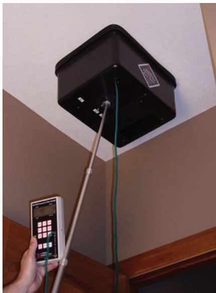
Figure 39.55(D) A technician measuring the airflow from an exhaust fan using an exhaust fan flow meter and digital gauge.
