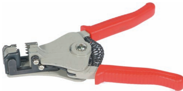
Figure 5.10 Wire stripping and crimping tools. (A) A combination crimping and stripping tool for crimping solderless connectors, stripping wire, cutting wire, and cutting small bolts. (B) An automatic wire stripper. Photos by Bill Johnson
