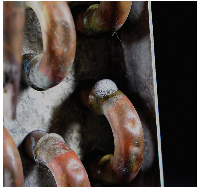
Figure 8.10 Foam “cocoons” of a microfoam solution on a small leak on the U-bends of a coil. Some microfoam solutions will detect and pinpoint leaks as small as 0.5 oz/year.
