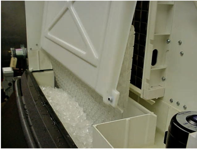
Figure 27.35 A full ice storage bin prevents the ice slab from closing the bin switch. Courtesy Ferris State University. Photo by John Tomczyk
