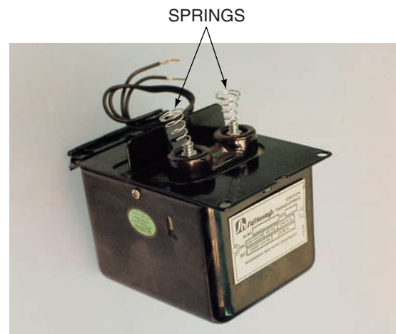
Figure 32.62 Springs on the secondary (high-voltage) winding of the ignition transformer. Photo by Bill Johnson
