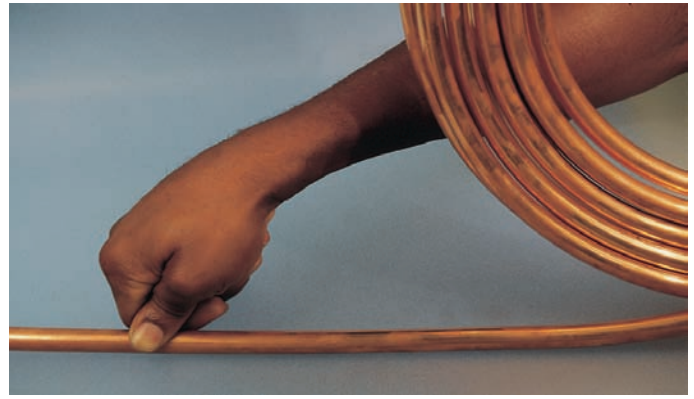
Figure 7.3 A roll of soft-drawn copper tubing. Place on a flat surface and unroll.
