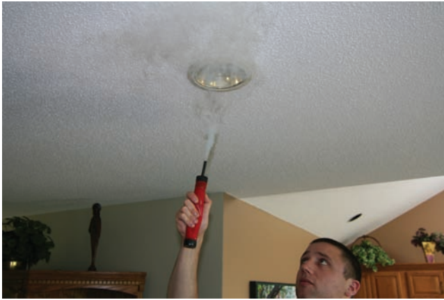
Figure 39.34 An auditor holding a chemical smoke generator up to a recessed light to find out if there is a possible air path to the outside. Courtesy Ferris State University. Photo by John Tomczyk
