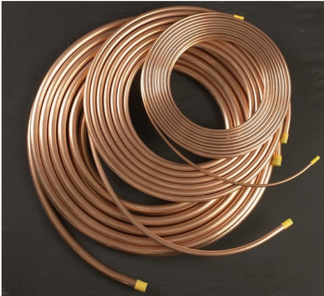
Figure 7.1 Soft-drawn copper tubing typically comes in 50-ft rolls. Note that the ends of the rolls are capped to keep the interior of the tubing clean.
