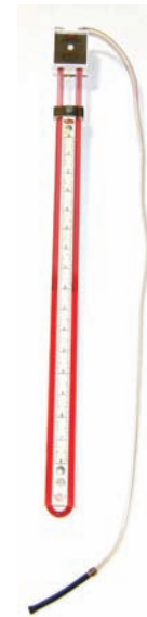
Figure 31.10 A manometer used for measuring pressure in inches of water column. Courtesy Ferris State University. Photo by John Tomczyk
