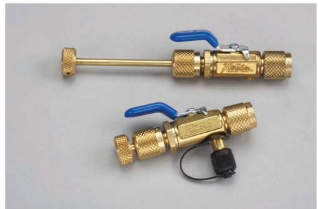
Figure 41.9 A hand valve used to press the Schrader valve stem and control the pressure. It can also be used to back the valve stem out. Backing the valve stem out while pulling a vacuum on a system causes less system restriction and a faster and more effective evacuation procedure. Courtesy Ritchie Engineering Company, Inc.
