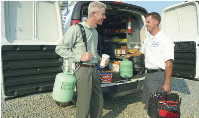
Figure 5.70 Carrying strap for carrying refrigerant cylinders on the ground or up a ladder. Courtesy SC Products, Inc., Wilmington, DE
