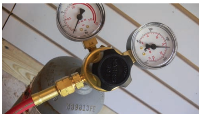
Figure 7.34 Pressure registers on the acetylene cylinder gauge.
