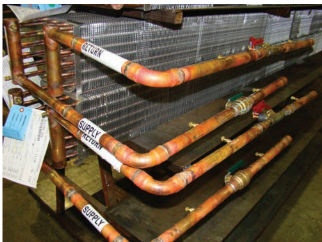
Figure 26.25(C) Evaporator coils piped for chilled glycol. Photo by Dick Wirz
