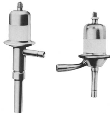
Figure 24.46 Automatic expansion valves. They resemble the TXV, but they do not have the bulb for sensing temperature at the suction-line end of the evaporator. Courtesy Singer Controls Division
