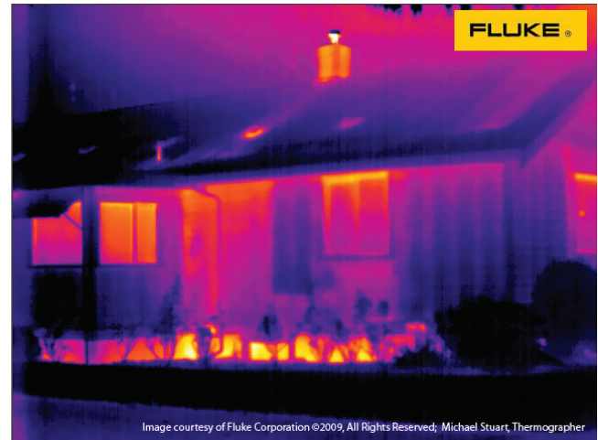
Figure 39.11(A) A thermal imaging camera showing heat escaping a building envelope. Courtesy Fluke Corporation
