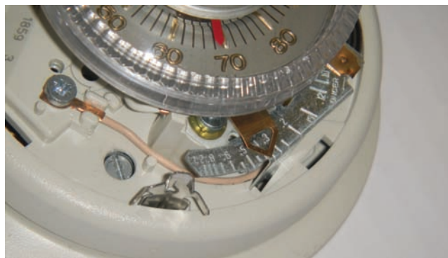
Figure 14.5 The heat anticipator as it appears in an actual thermostat. Photo by Eugene Silberstein
