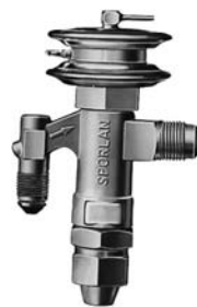
Figure 24.32 A pressure-limiting expansion valve. When the pressure is high in the evaporator, such as during a hot pulldown, this valve will override the thermostatic element with a pressure element and throttle the refrigerant. Courtesy Sporlan Valve Company
