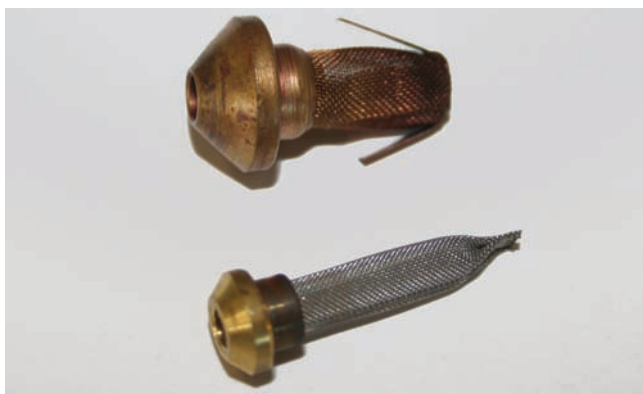
Figure 24.9 Most valves have some sort of inlet screen to strain any small particles out of the liquid refrigerant before they reach the very small opening in the expansion valve. Courtesy Ferris State University. Photo by John Tomczyk
