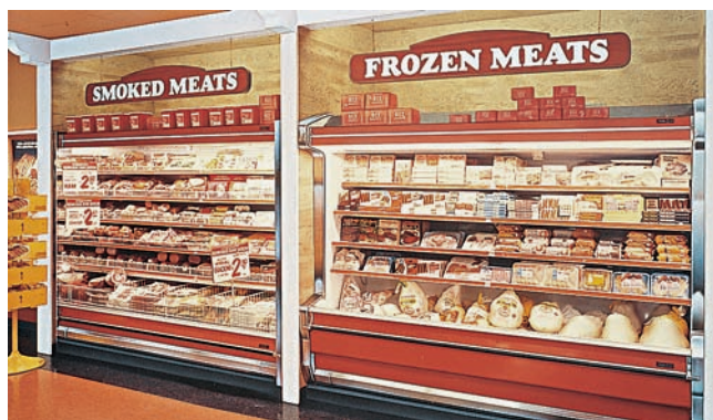
Figure 26.3 This self-contained refrigerated box has its condensing unit built-in. Refrigeration tubing does not have to be run. This box rejects the heat it absorbs back into the store. It is movable because it needs only an electrical outlet and, sometimes, a drain, depending on the box. Courtesy Hill Refrigeration
