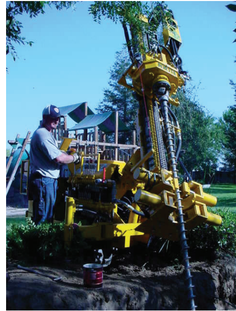
Figure 44.41 Diagonal drilling rig showing small-bore drilling equipment. Courtesy Earthlinked Technologies, Inc.
