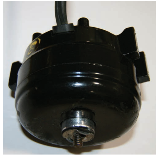
Figure 19.19 A small condenser fan motor that does not pull enough amperage at locked-rotor amperage (LRA) to create enough heat to be a problem. This is known as impedance motor protection. Courtesy Ferris State University. Photo by John Tomczyk
