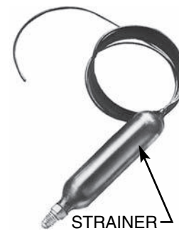
Figure 29.31 A capillary tube metering device with the strainer at the inlet. This strainer is soldered into the line and is not easy to service. Courtesy Parker Hannifin Corporation
