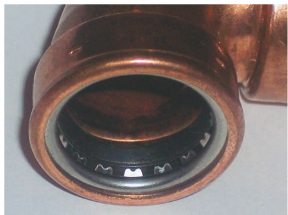
Figure 7.79 Push-on fitting with internal gasket and metal teeth for grabbing onto the pipe section.
