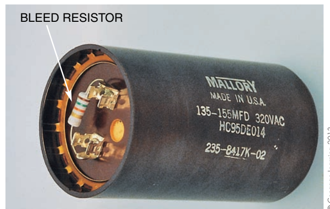
Figure 20.26 A start capacitor with a bleed resistor across the terminals to bleed off the charge during the off cycle. SAFETY PRECAUTION: Make certain that capacitors are completely discharged before you come into contact with the terminals. • Photo by Bill Johnson
