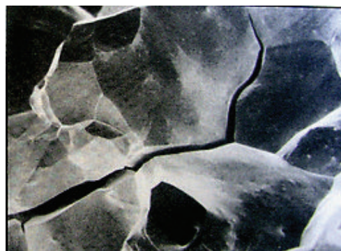
Figure 8.1 Electron micrograph of a “clean” silver soldered joint. Note the crack lines and other impurities of the metal. Further magnification shows actual metal separation.
