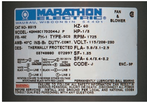
Figure 18.2 A motor nameplate. Photo by Bill Johnson
