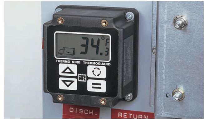
Figure 28.16 An alarm may alert the driver if the load's condition is not being maintained. Courtesy Thermo King Corp.
