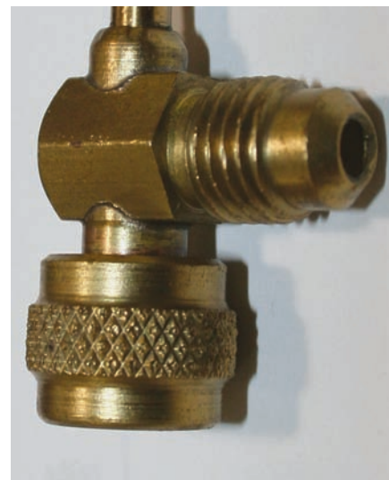
Figure 8.54 This small valve can also be used for controlled gauge readings. To read a pressure in a Schrader port, the adapter valve may be used by turning the valve handle.
