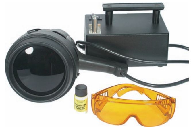
Figure 3.39 Common methods used for leak detection. (A) Listening for audible leaks. (B) Ultrasonic leak detector. (C) Soap-bubble solution. (D) Soap-bubble solution causing bubbles to form when a leak is present. (E) Halide torch. (F) The flame on the halide leak detector turns green when a leak is present. (G) Electronic leak detector. (H) Ultraviolet leak detection equipment.
