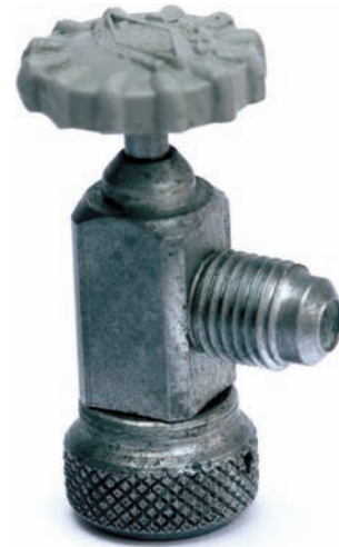
Figure 8.53 This gauge adapter can be used instead of the gauge depressors that are normally in the end of the gauge lines. The adapters may be used for gauge readings. Photo by Bill Johnson
