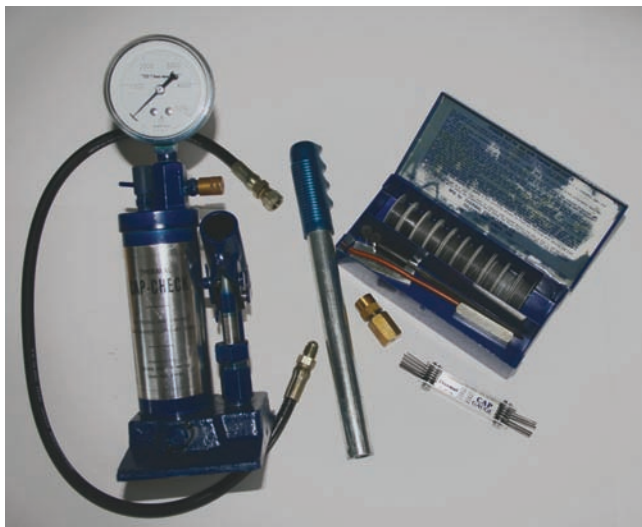
Figure 24.51 Hydraulic capillary-tube cleaning kit. Courtesy Ferris State University. Photo by John Tomczyk
