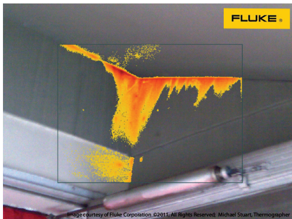
Figure 39.28 A thermal imaging camera showing warm air exfiltrating above a door. Courtesy Fluke Corporation
