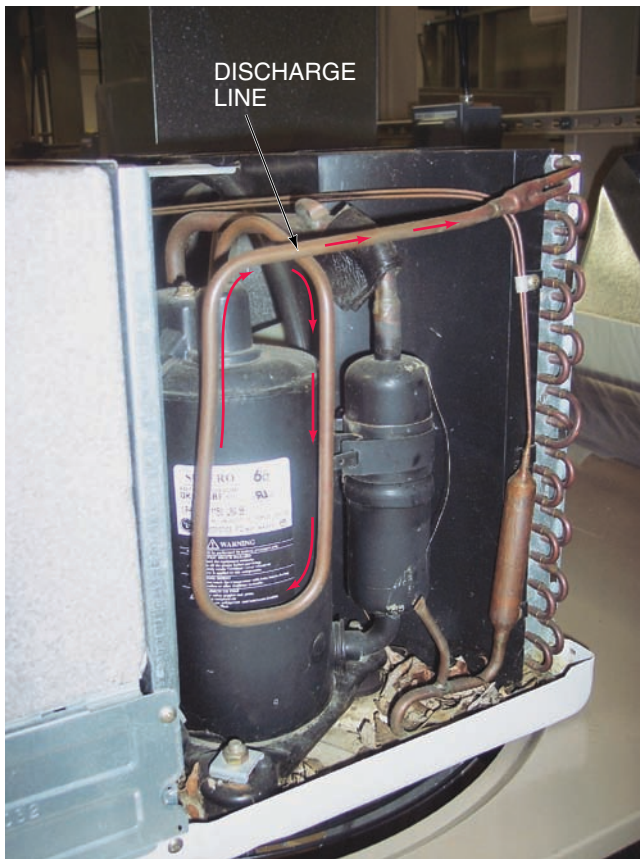
Figure 3.32 The discharge line connects the outlet of the compressor to the inlet of the condenser.
