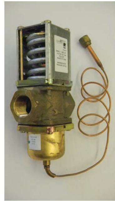
Figure 14.61 This valve maintains a constant head pressure for a water-cooled system during changes in water temperatures and pressures. Photo by Eugene Silberstein
