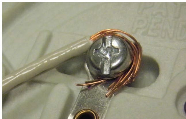
Figure 6.47 Stranded wire should not be directly connected under a screw terminal. Photo by Eugene Silberstein
