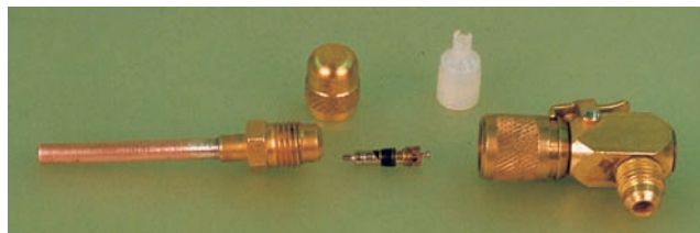
Figure 45.131 Remove the Schrader valve depressors from gauge lines and use the special fitting on the right to depress the valve cores. Photo by Bill Johnson
