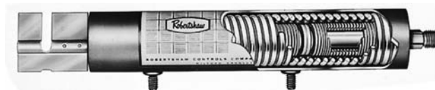
Figure 22.41 A piston-type shutter operator. The high-pressure discharge gas is on one side of the bellows, and the atmosphere is on the other side. When the head pressure rises to a predetermined point, the shutters begin to open. In the summer, the shutters will remain wide open during the running cycle. Courtesy Robertshaw Controls Company
