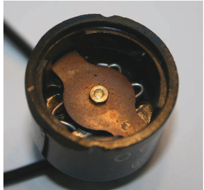
Figure 14.23 A motor temperature-sensing thermostat. Courtesy Ferris State University. Photo by John Tomczyk
