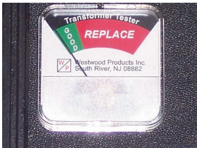
Figure 32.65 Display of an ignition transformer tester. Courtesy Oilheat Associates, Inc. Photo by John Levey
