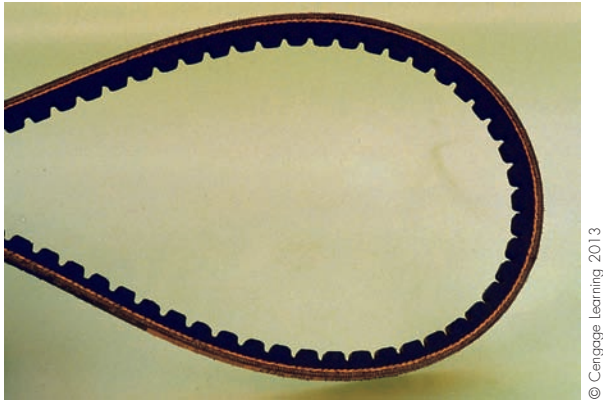
Figure 18.41 This belt with grooves has a tractor-type grip. Photo by Bill Johnson
