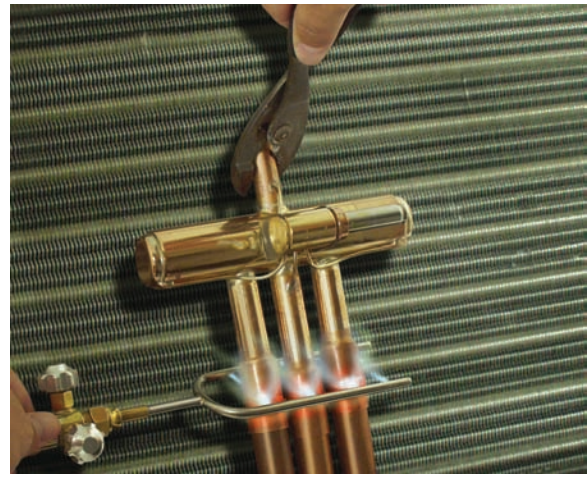
Figure 43.11 (A) Specialized torch tip designed for removing reversing valves. (B) Using the torch tip. Photos courtesy Uniweld Products, Inc.
