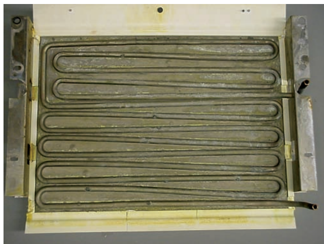
Figure 27.21 A serpentine coil soldered to the back of a cell-type ice cube evaporator. Courtesy Ferris State University. Photo by John Tomczyk
