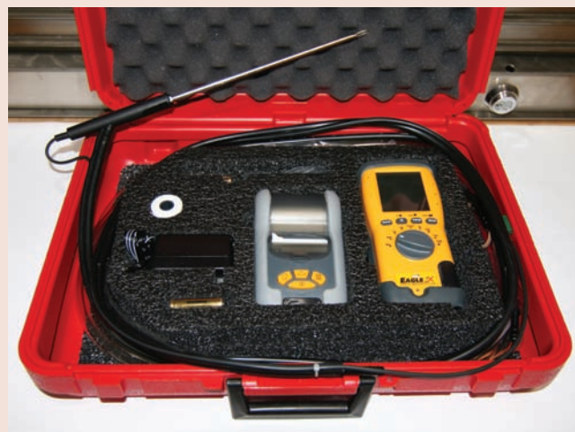
Figure 31.112 Modern digital furnace efficiency testing equipment. Courtesy Ferris State University. Photo by John Tomczyk
