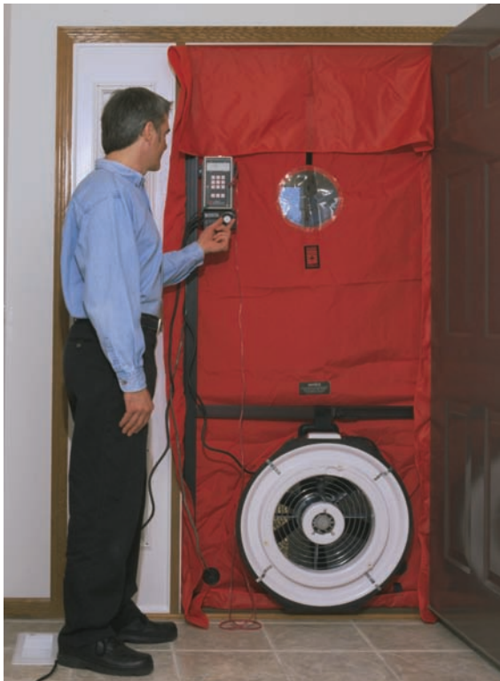
Figure 5.80 A technician performing a blower door test on a residence dwelling. Courtesy of The Energy Conservatory
