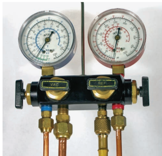
Figure 8.57 (A) A gauge manifold with copper gauge lines and a large vacuum pump line. (A) Photo by Bill Johnson ( Continued )
