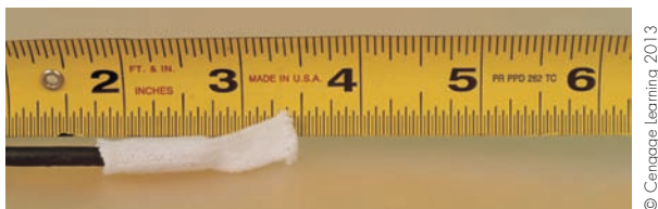
Figure 41.16 This electronic thermometer temperature lead has a damp cotton cloth wrapped around it to convert it to a wet-bulb lead. Photo by Bill Johnson
