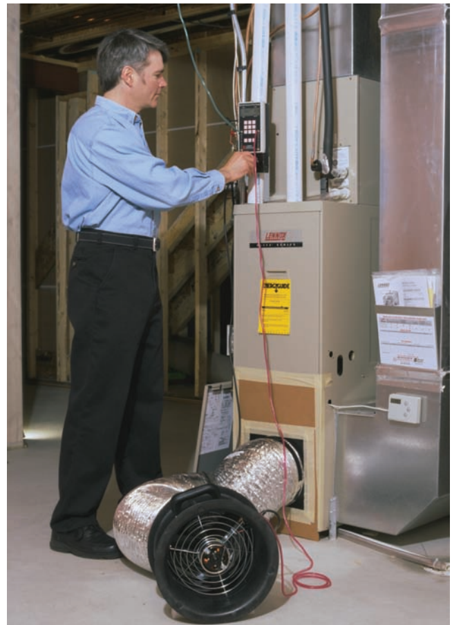
Figure 5.81 A technician performing a duct pressurization test on a residential furnace. Courtesy of The Energy Conservatory
